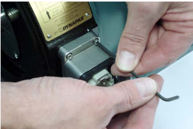
7.2 Secure the Sensor Module with (4) #6 X 32UNC screws. Tighten to a nominal 5in-lbs.
