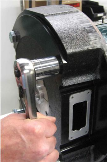
2.5 Position the Pulsewheel to its correct position under the sensor modules by sliding the shaft adapter along the shaft until the front face is flush cover surface of the housing. The clamp screws may need to be loosened to allow easy sliding.
