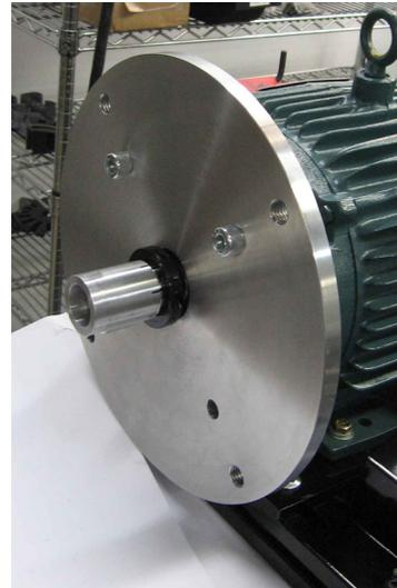
2.2 Slide Pulsewheel onto the shaft. Leave it loose at this time. Anti-seize may be used on the shaft & C-face to reduce future corrosion
