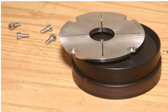
1.3 Loosely insert 4 M5 screws in the notches of the clamp into the shaft adapter face. Do not tighten at this time. The wheel is ready to install.
