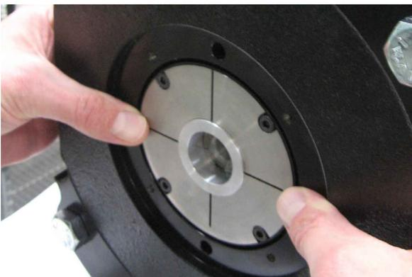
2.6 Tighten Shaft Clamp's 4, M5X.0.7M Screws in a star pattern (~35 in-lbs, 90in-lbs max) to engage the clamp in the correct position.
