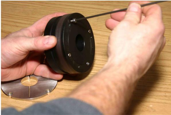
1.2 Insert Clamp plate into the face of the Shaft adapter. The "V" shape of the parts will nest into one another.
