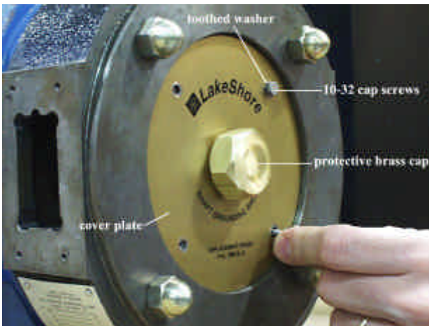
Figure 8: Securing the Holder/Cover Plate Assembly
