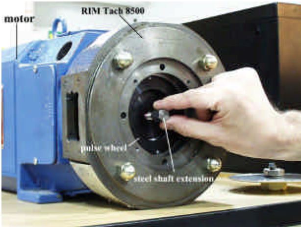
Figure 7: Installation of Shaft Extension
