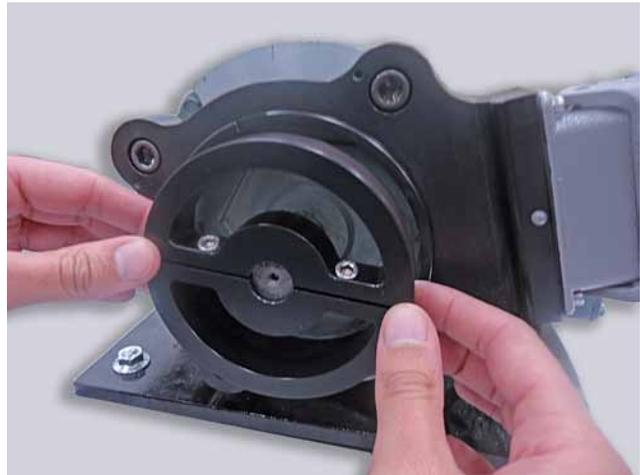
**6.0 Position the wheel such that its front surface is flush with housing groove surface.**
