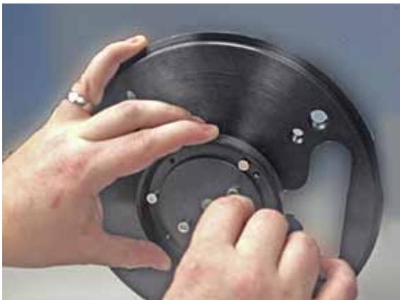
Tighten to the appropriate torque for the particular screw size of the motor. Use of “Low Strength” thread-locker is suggested.
