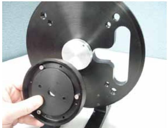
Orient the Shaft adapter to end of the motor. The fit should be snug, but smooth.
