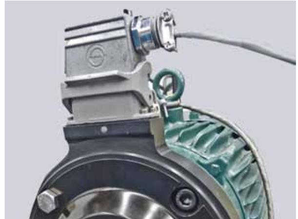
**9.0 Grab mating connector, unscrew (4) mating connector screws.**
