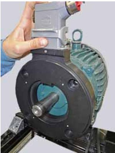
**6.0 Position the wheel such that its front surface is flush with housing groove surface.**
